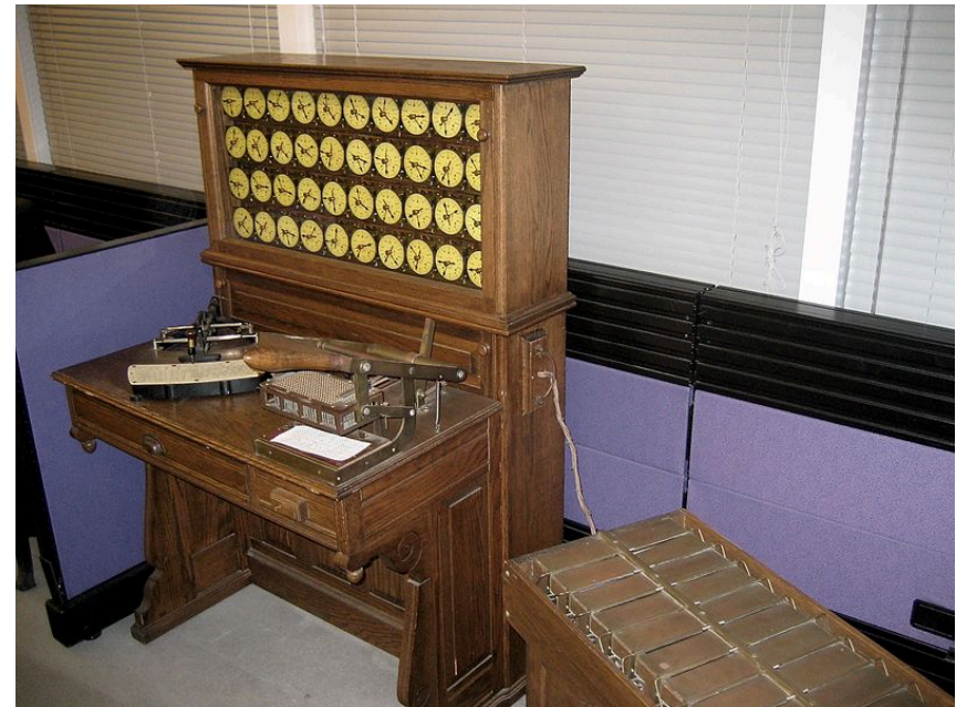
Hollerith 1890 tabulating machine & sorting box. By Adam Schuster - Flickr: Proto IBM, CC BY 2.0, https://commons.wikimedia.org/w/index.php?curid=13310425
